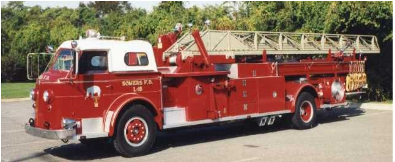
Ladder 18 at Lincolndale Firehouse parking lot after re-painting and a fiberglass cab roof installed
